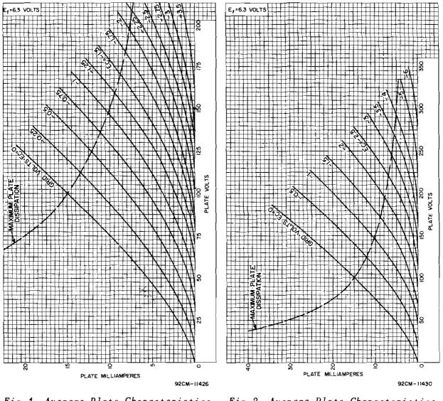
Fig. 1 - Average Plate Characteristics for Type 8058.
