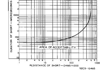
Fig. 4 - Thyratron-Type Shorts Test for Type 8058.
